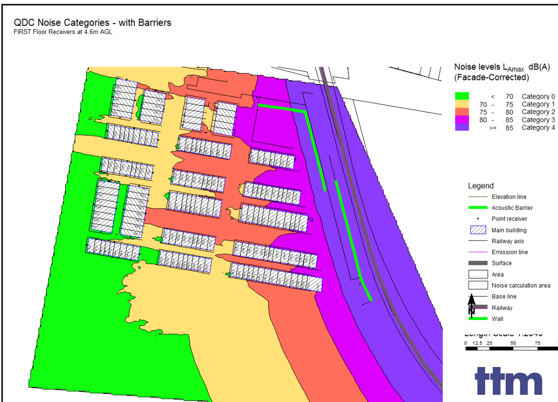
Figure 7: Predicted L_{Amax} Rail Noise Levels – First Floor
