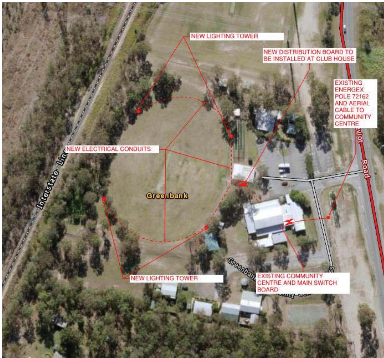
Image 2.2.1 Electrical Infrastructure and Proposed Upgrade
