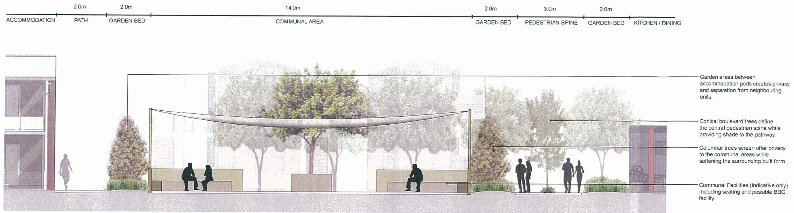
SECTION 5 - TYPICAL COMMUNAL AREA
