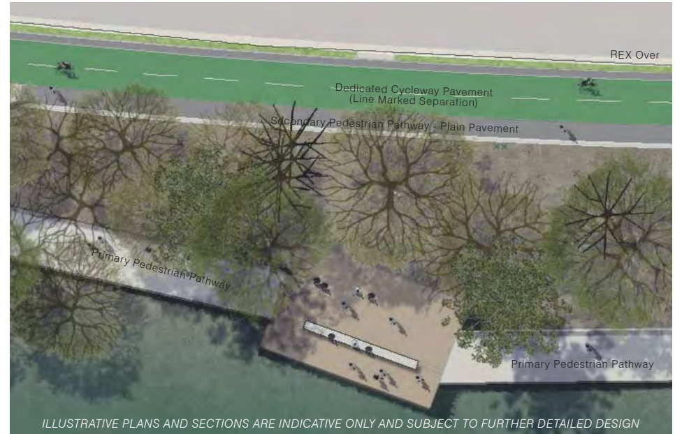
Figure 5.48: Goodwill Extension Type 2 Typical Pavement Treatment
