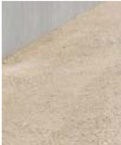
Stabilised Decomposed Granite
