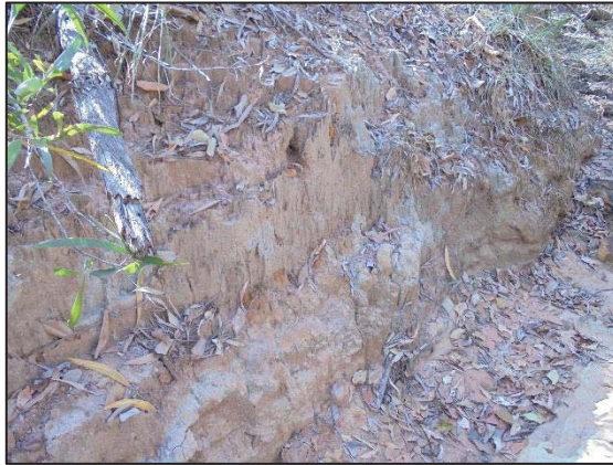
Image 5. Minor tunnel erosion to bank edge
