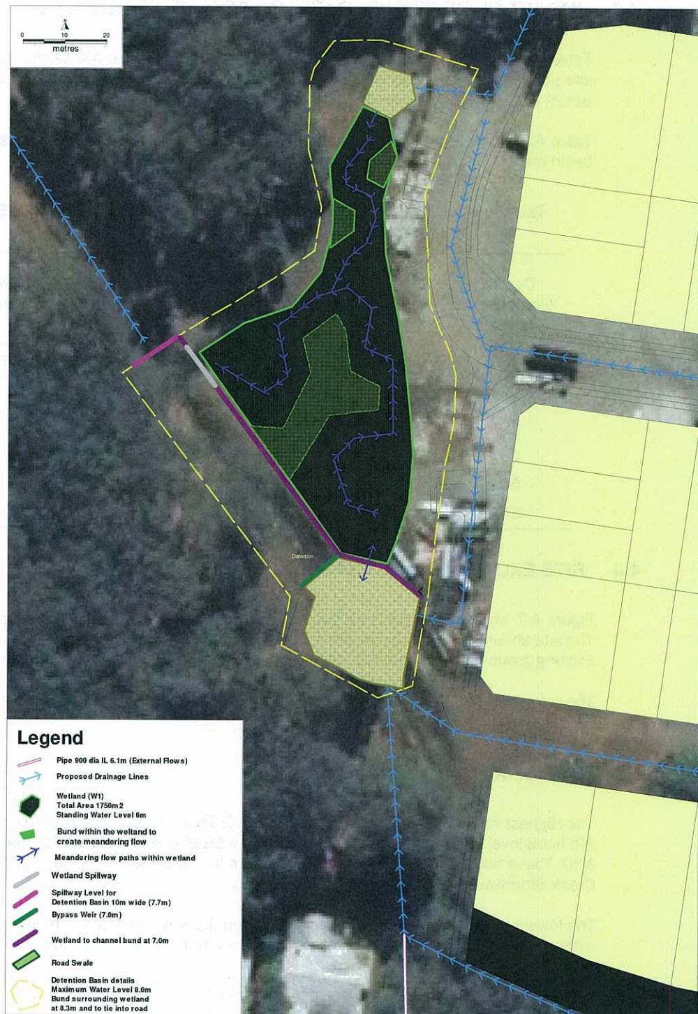
Figure 4.2 Wetland/Detention Basin Details
