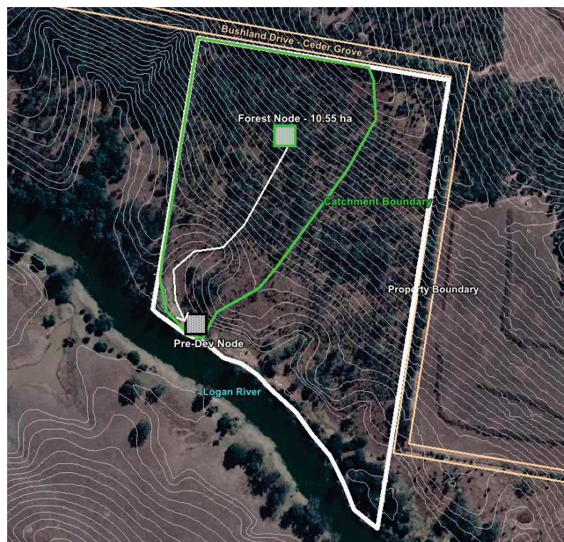
Figure 3 MUSIC Model Setup Schematic Diagram – Existing Case
