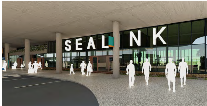
IDT-3 TENANT HAMPER SIGN (SEALINK) Wall mounted 3D fabricated alu. letters, illuminated facelit acrylic or translucent graphics on opal min 100mm deepd. Approx size 19000x1800mm (11.25sqm)
