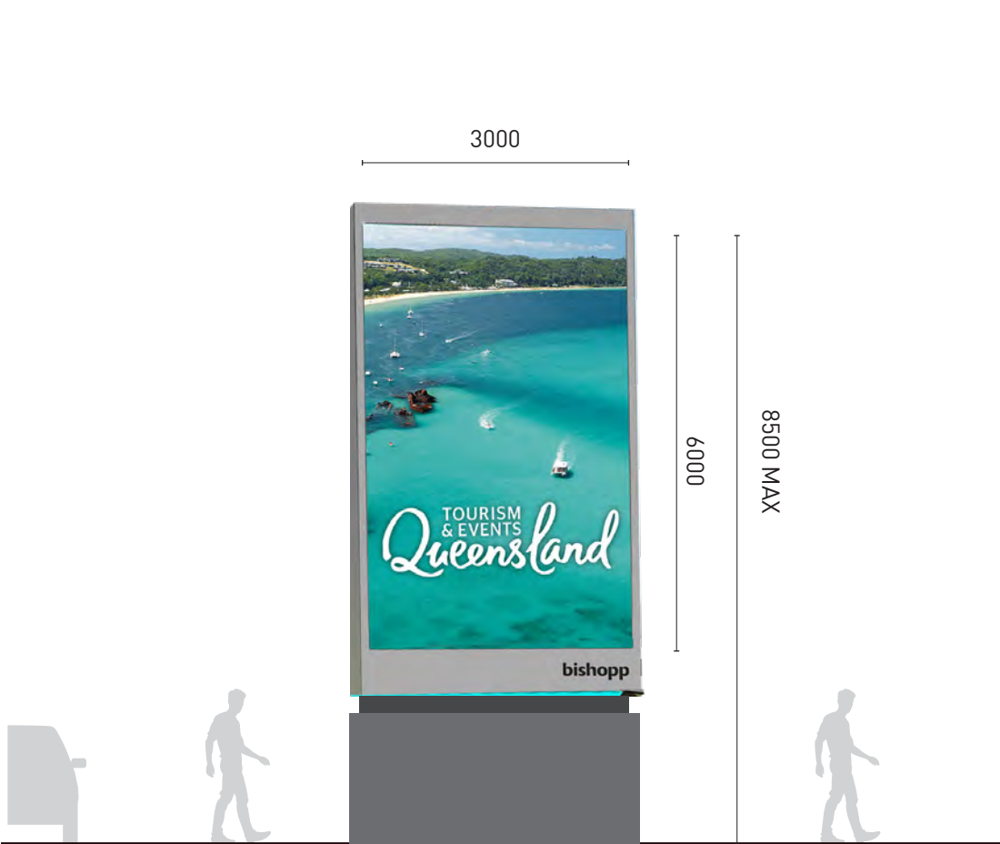
EB-1 ELECTRONIC BILLBOARD - CHANGEABLE CONTENT Double sided digital display sign on solid base Screen Size: 3000x6000mm (18sqm) Overall sign size: approx 8500mm high
