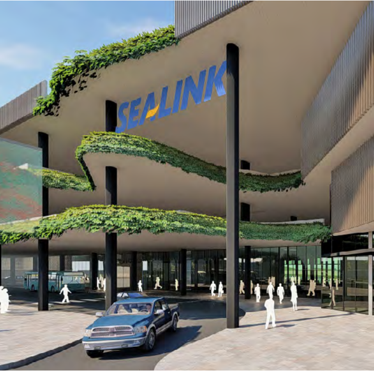
IDT-1 and IDT-2 TENANT UNDER AWNING SIGN (SEALINK) 2x 3D fabricated sign to tenants guidelines or 2 x 3D fabricated alu. letters illuminated facelit acrylic or translucent graphics on opal min 200mm deep Approx size 5800x1900mm each (11sqm)
