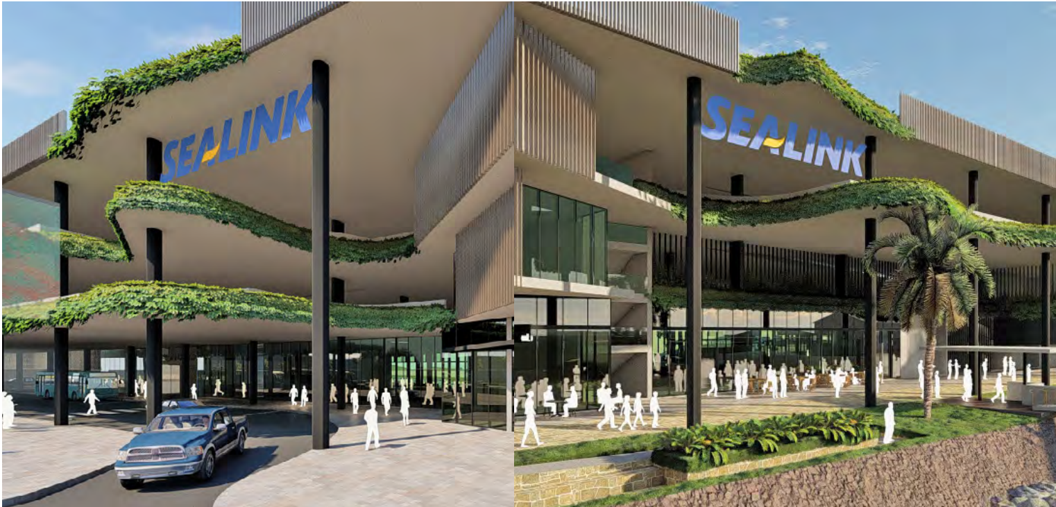
SEALINK IDT-1 and 2 2x 3D fabricated alu. illuminated backlit letters min 200mm deep Sign to tenants guidelines or 2 x 3D fabricated alu. letters illuminated facelit acrylic or translucent graphics on opal min 200mm deep Approx size 5800x1900mm each
