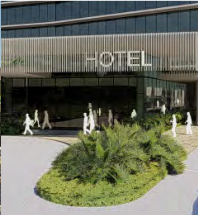
HOTEL IDT-3 Backlit fabricated letters, Powdercoated aluminium. Wall mounted 3D fabricated backlit alu sign. Design subject to confirmation of hotel brand. Approx size 5200x1200mm
