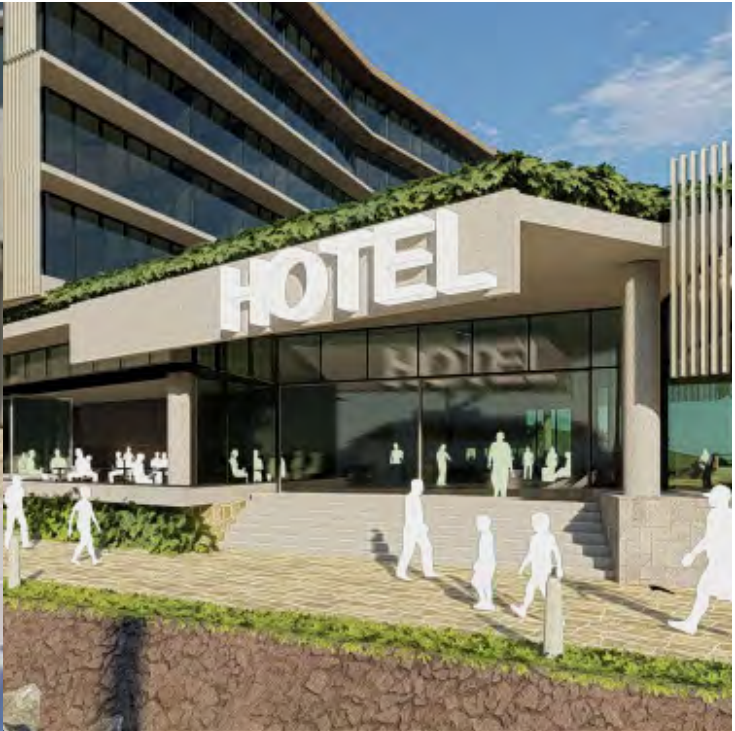
HOTEL IDT-4 Backlit fabricated letters, Powdercoated aluminium. Wall mounted 3D fabricated backlit alu sign. Design subject to confirmation of hotel brand. Approx size 5200x1200mm
