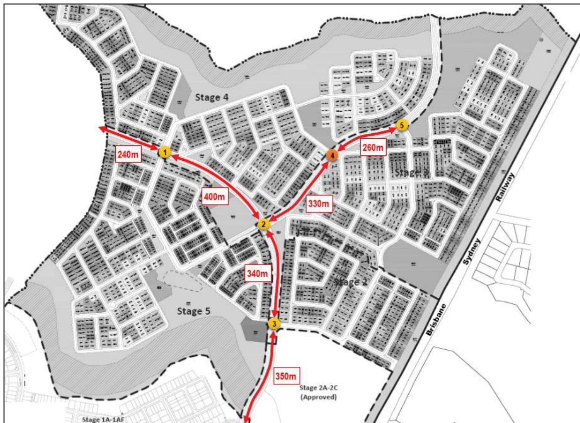
Figure 4.3: Stages 2-5: Key Intersection Spacing
