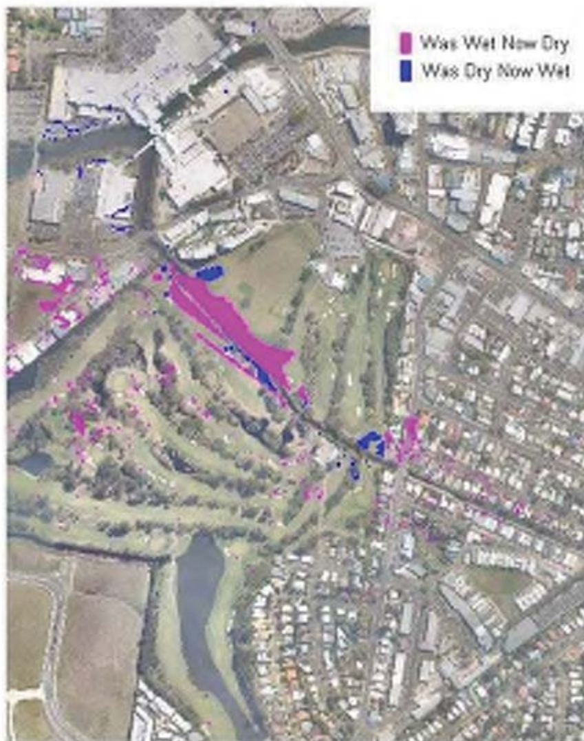
Image 2 1% AEP Stage 1 Temporary Works Flood Impact
