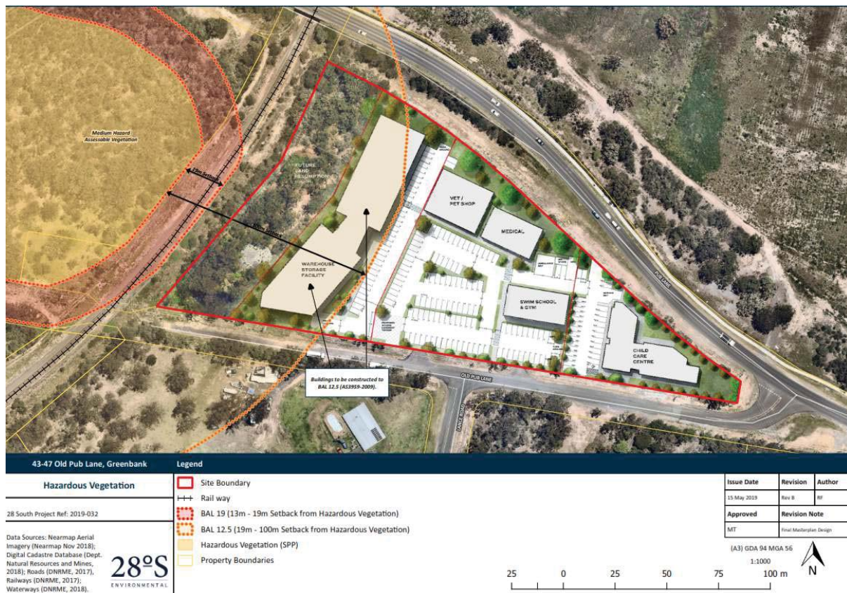
Figure 1: Proposed Concept Plan with bushfire hazard setbacks (28 South Environmental, 2019)
