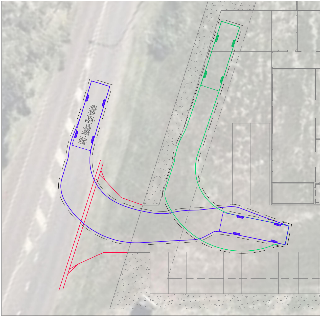
MRV LOADING BAY - ENTRY
