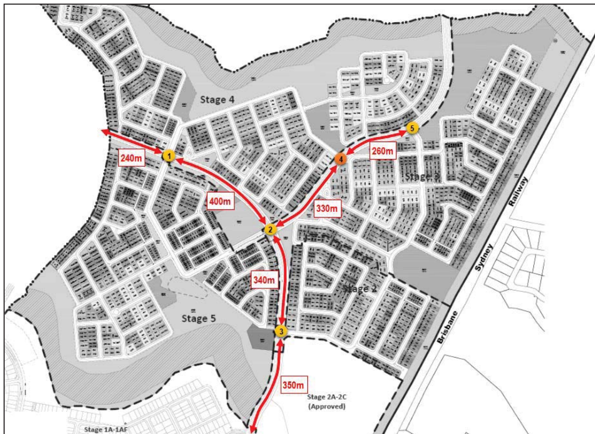
Figure 4.3: Stages 2-5: Key Intersection Spacing
