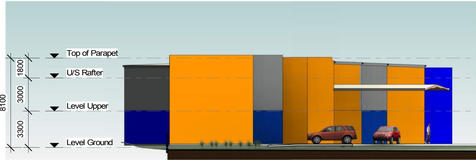
3 BUILDING 4 - SOUTH ELEVATION 1 : 200
