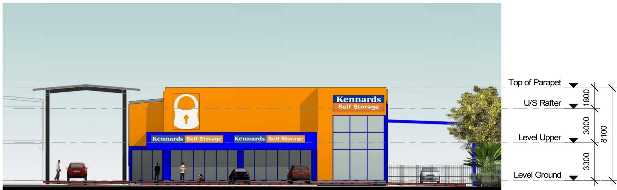
4 BUILDING 1 - SOUTH ELEVATION 1 : 200
