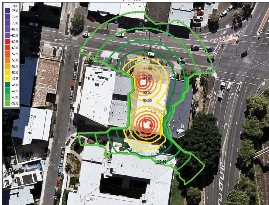
Plate B2: Noise contours at 7.6m. Levels are in dB(A) L_{eq,1hr}
