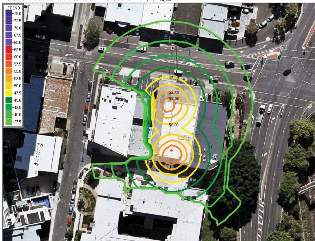
Plate B3: Noise contours at 10.6m. Levels are in dB(A) L_{eq,1hr}
