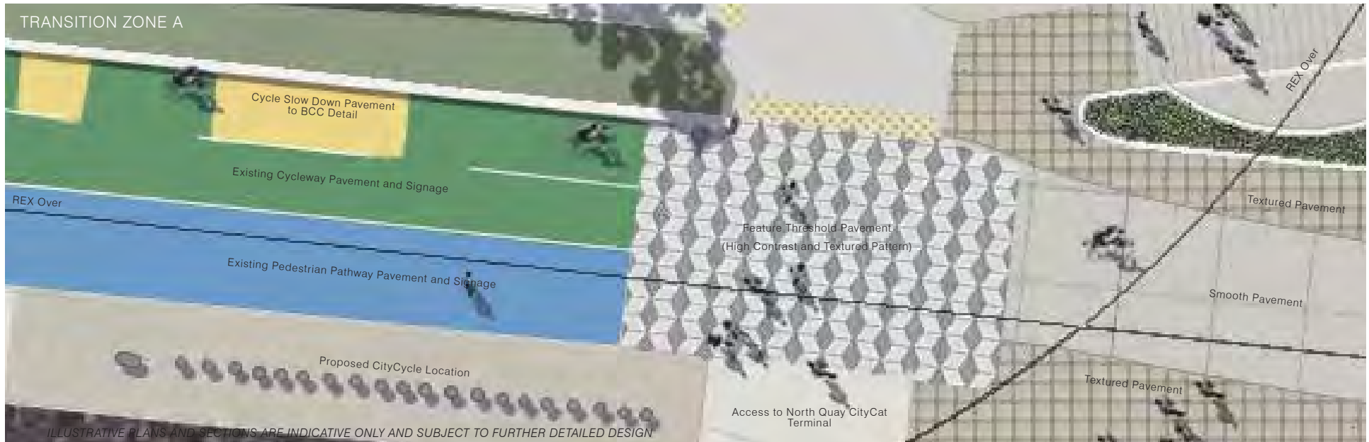
Figure 5.52: Transition Zone A Typical Pavement Treatment
