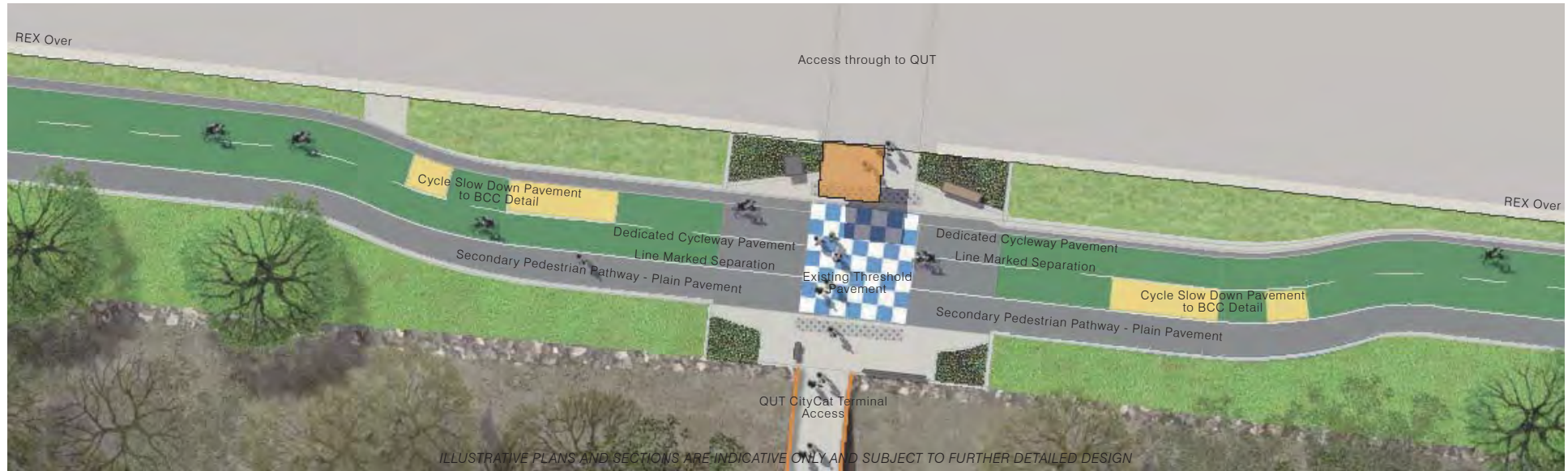
Figure 5.57: Transition Zone E Typical Pavement Treatment
