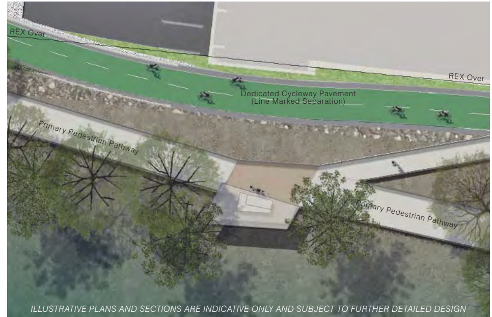
Figure 5.46: Goodwill Extension Type 1 Typical Pavement Treatment
