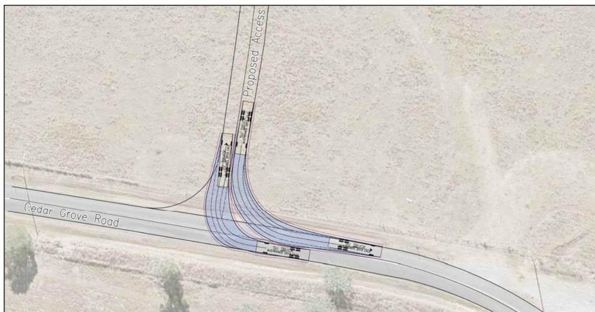
Figure 2.4 Proposed access road intersection
