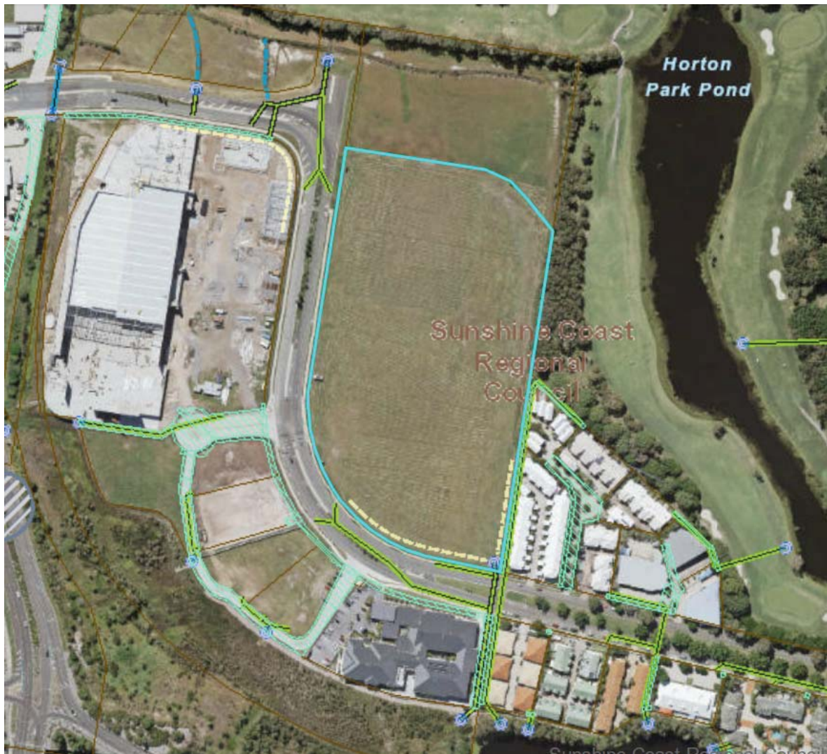
Figure 2-1 Existing Site Drainage (SCC MyMaps)
