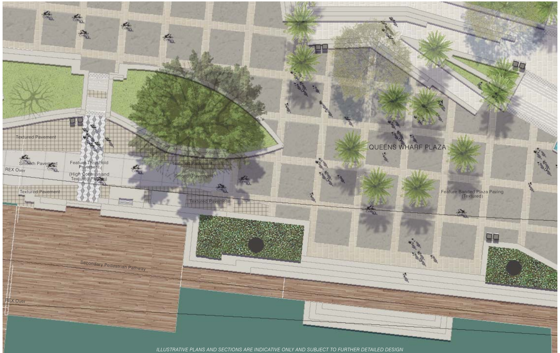
Figure 5.54: Transition Zone B Typical Pavement Treatment
