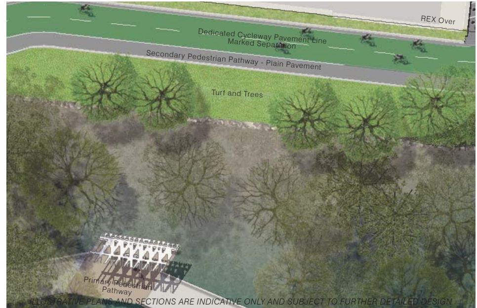
Figure 5.50: Goodwill Extension Type 3 Typical Pavement Treatment
