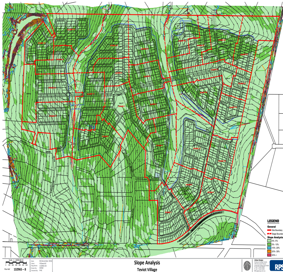
Figure 4a: Slope analysis north of Pub Lane with light and dark green areas representing slopes of 0-5%, and 5-10% respectively. The neighbouring area in the north west with steep slopes is the sparsely vegetated slopes of the lagoon (Refer Figure 4b ).
