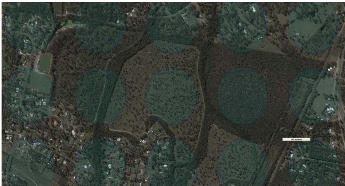
Figure 5a: GIS 200m diameter 'circular assessment areas' linked to 1km squares to UTM Grid as per the CSIRO GIS database.
