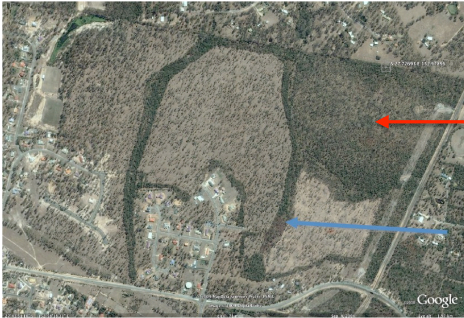
Figure 2a: Arrow (blue) showing example of interface on boundary along Stages 2 & 5 with linear parkland vegetation i.e. RERE conservation landscape < approximately 60m width. Arrow (red) shows the larger vegetated area in the NE, which is isolated from offsite vegetation by clearing. If this area is not initially cleared, a 33m fire break will need to be maintained on any advancing development boundary.
